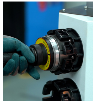
Quick-change system for easy replacement of die molds
