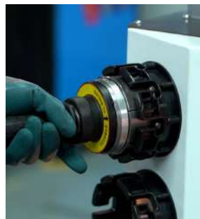
Quick-change system for easy replacement of die molds
