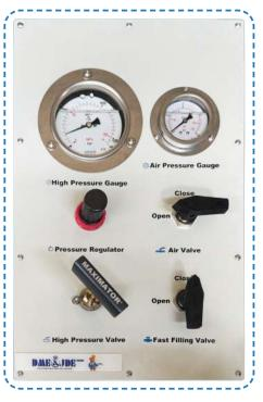
The pressure testing bench control panel is used to manage and monitor the pressure testing process, including setting pressure values, starting tests, and viewing test results.
