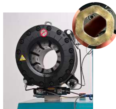
Crimper Dies Type Hexagonal Crimping Scheme (Popular)
