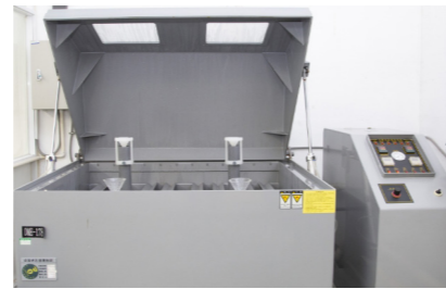
Salt Spray Testing
