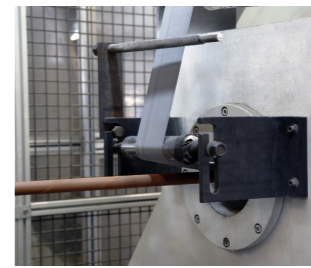
Fiber Reinforcement Wrapping
