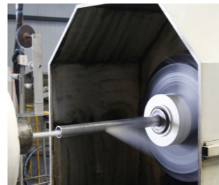
Fiber Reinforcement Wrapping
